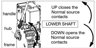
Figure 1-8. Normal (lower shaft) operation on 150–600 amp. J–design transfer switches..
